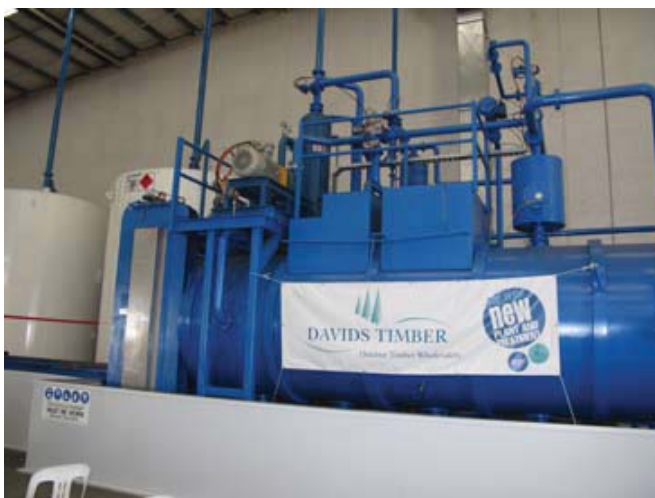
State-of-the-art .. new LOSP plant at Dauids Timber – a dual operation capable of treating both H3 LOSP green or water-based Determite H2F Blue.
